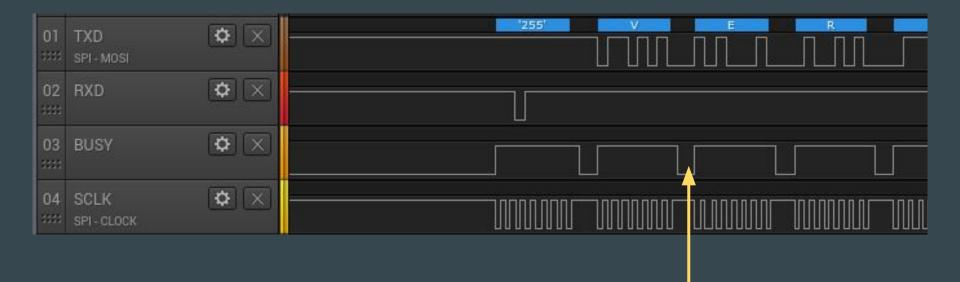
An PIN unlock request does not result in any immediate success/failure transmission, but...
