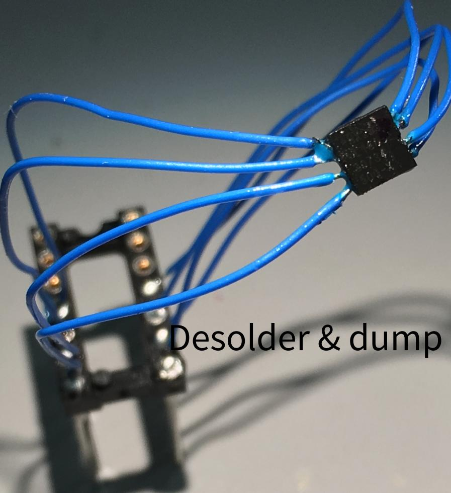
Desolder & dump the SPI flash \(^^)/
