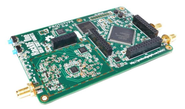
10 MHz to 6 GHz 20 MHz bandwidth (20 Msps quadrature) Half-duplex SDR transceiver
